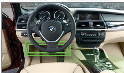
common location of OBD connectors
